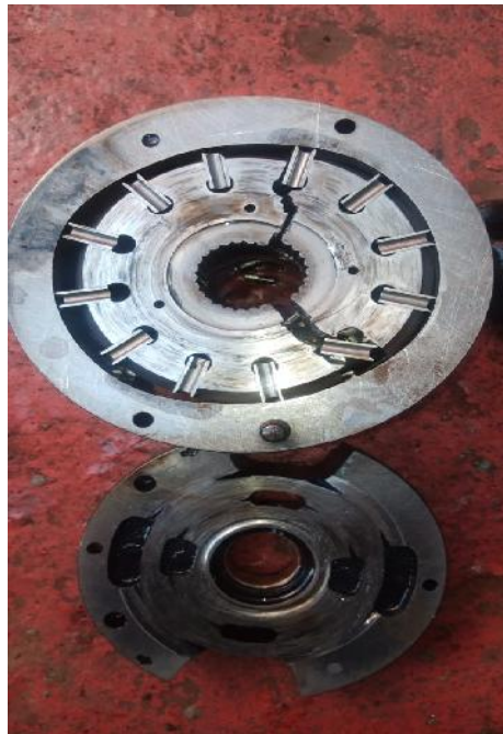
Gambar 11. Cartridge Pump Crane Rusak
